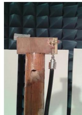
Figure. 11. Designed antenna into anechoic chamber.
